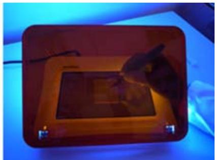
**Note:** For cutting fluorescent samples out of the gel, please lift the lid to access the gel.
